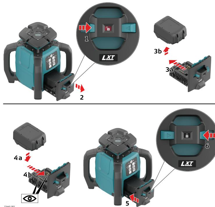
1. Always switch off the SKR001 before installing or removing of the battery tray.
