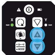
3. Press the X/Y Mode button to change to Y-axis.
