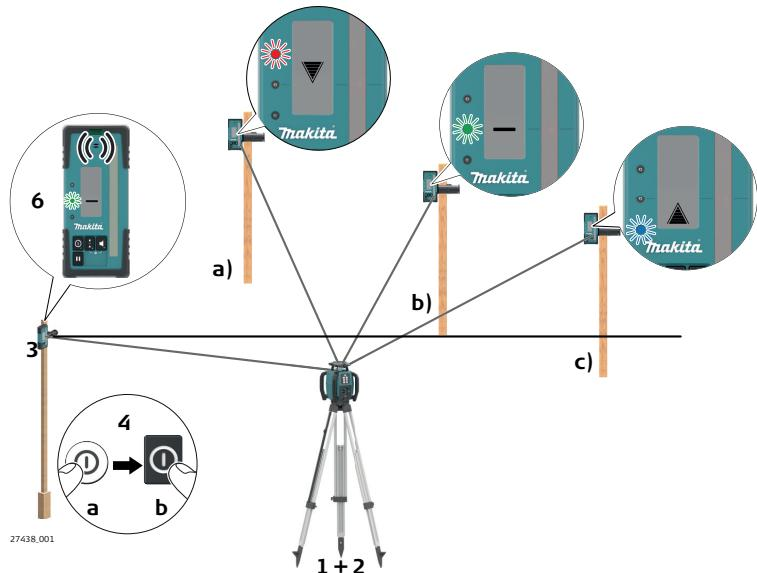
1. Set up the SKR001 on a tripod.
