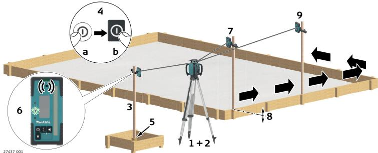
1. Set up the SKR001 on a tripod.
