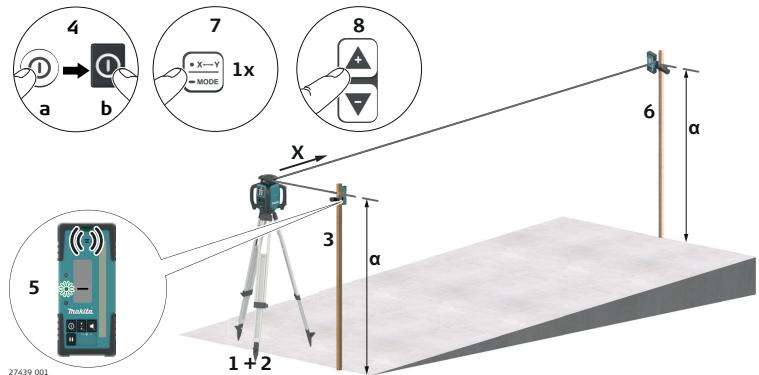
1. Set up the SKR001 on a tripod.
