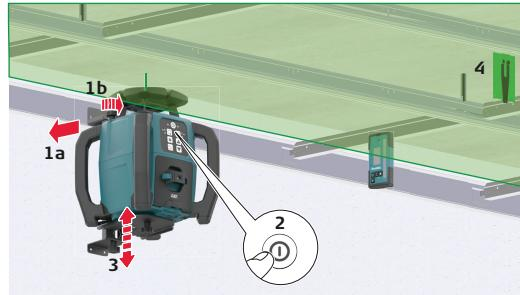
1. After mounting the first strip of ceiling trim at the desired height (centre position of the Target plate) below, attach the wall mount bracket and laser to the trim. Tighten the locking knobs on the top of the bracket.
